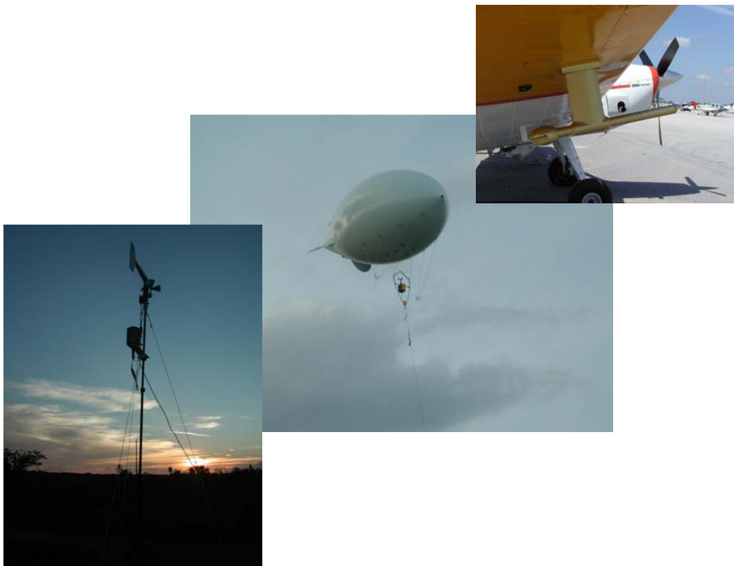
Figure 12. Meteorological support for the aerial trials included a surface tower, Kitoon and AIMMS-20
