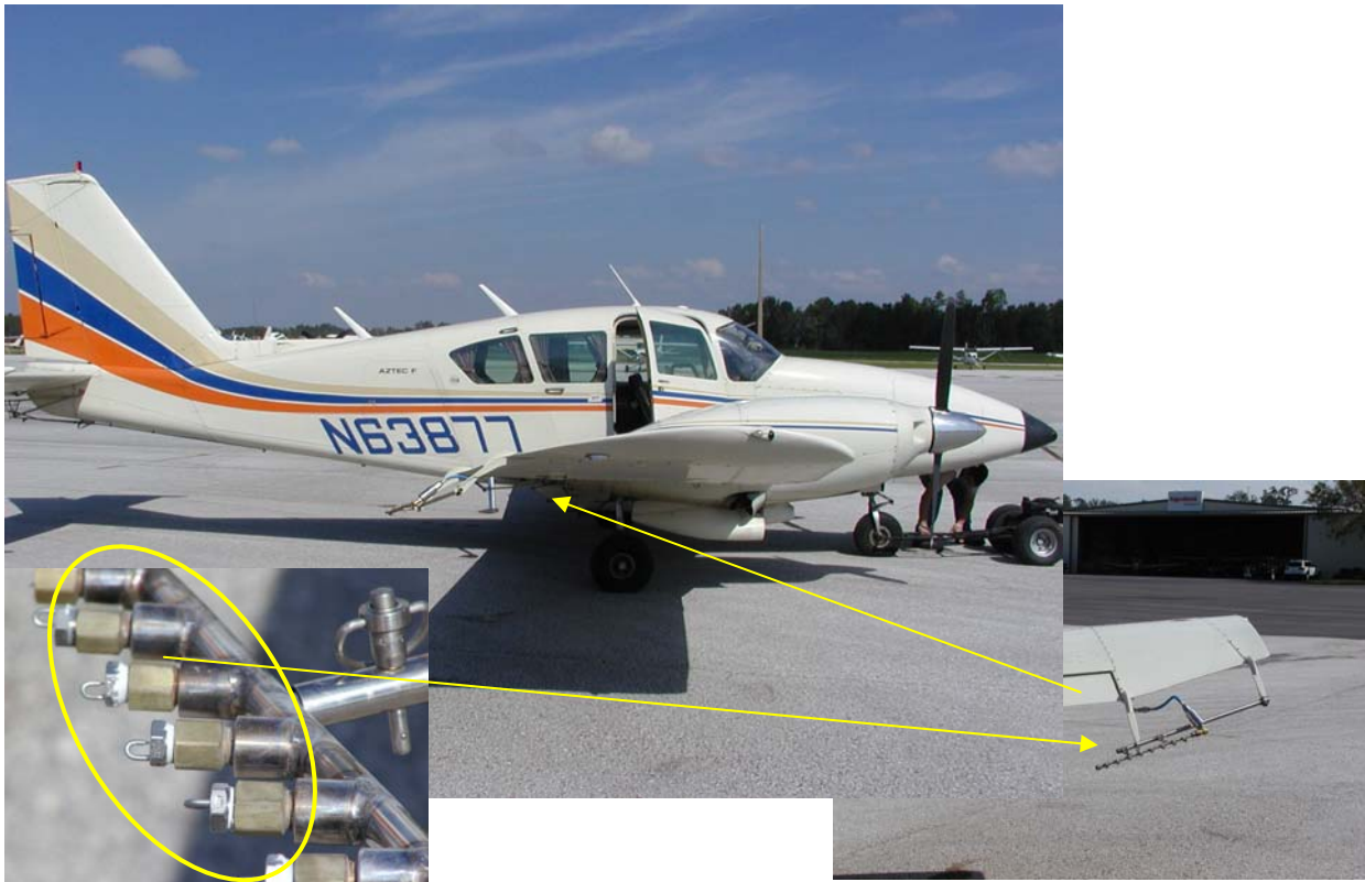
Figure 6. PCMCD Aztec with nozzle array mounted on starboard wing tip. Insert shows close-up of the 6-PJ20 HP nozzles
