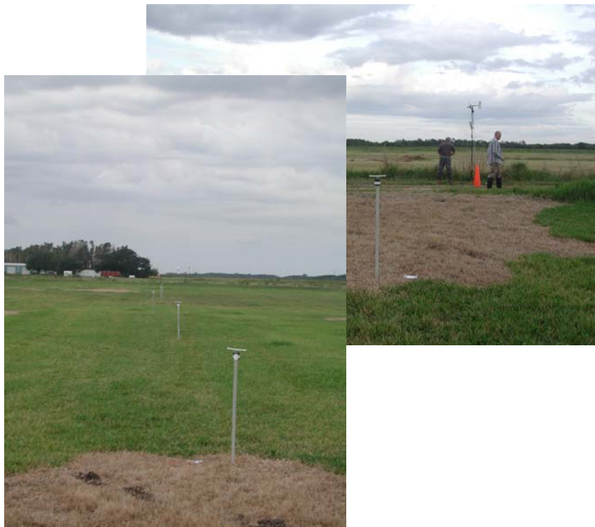
Figure 8. Fetch upwind and sample line downwind of spray line along gravel road in sod farm
