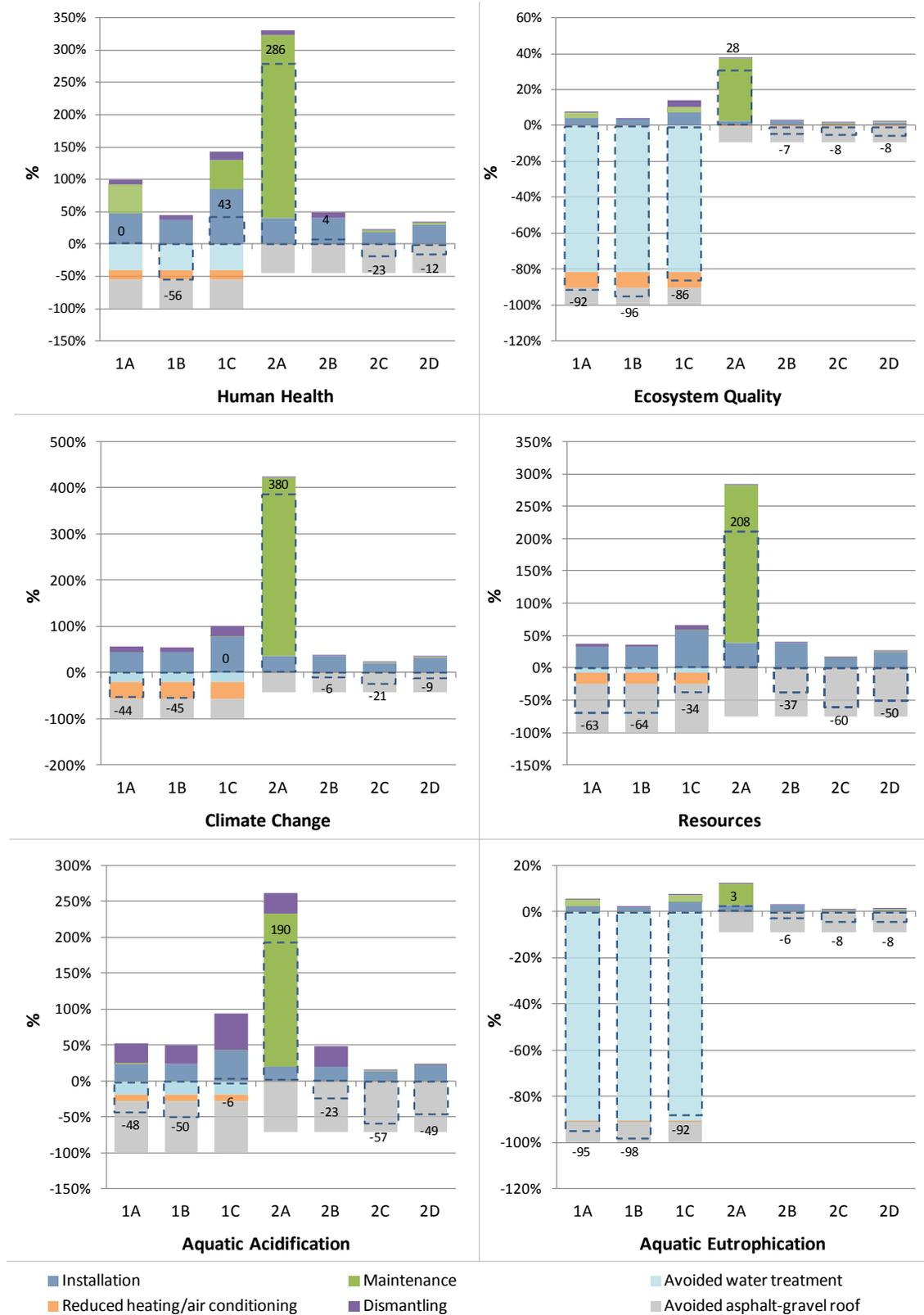
1A. Green roof (45 years, chemical fertilization as needed)      2A. Elastomeric membrane (25 years, reflective coating every 5 years)
